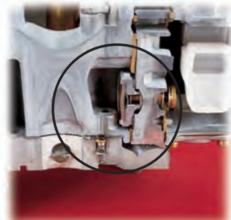
Cut-away of power valve blow-out protection.
